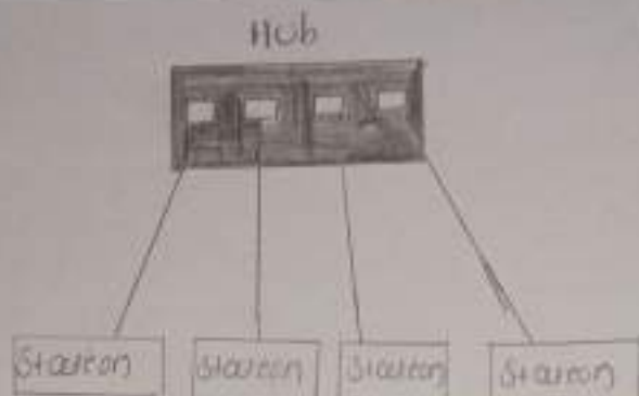
Figure 1.6 A star topology connecting four stations
