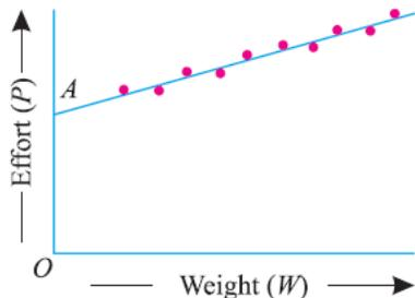
Mathematically, the law of a lifting machine is given by the relation :  $P = mW + C$
