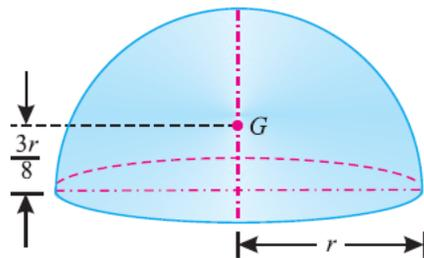
The centre of gravity of a hemisphere is at a distance of  $\frac{3r}{8}$  from its base measured along the vertical radius.
