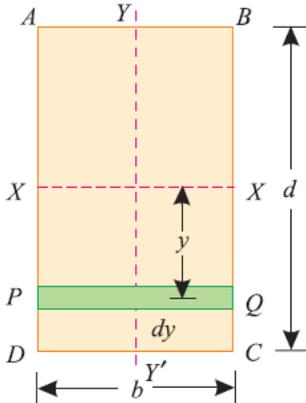
$$I_{xx} = \int_{-d/2}^{+d/2} b y^2 dy = b \int_{-d/2}^{+d/2} y^2 dy = b \left[ \frac{y^3}{3} \right]_{-d/2}^{+d/2} = \frac{bd^3}{12}$$
