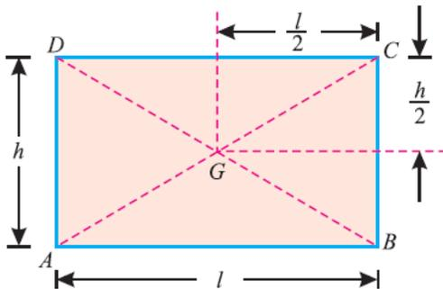
The centre of gravity of a rectangle (or a parallelogram) is at the point, where its diagonals meet each other. It is also a middle point of the length as well as the breadth of the rectangle
