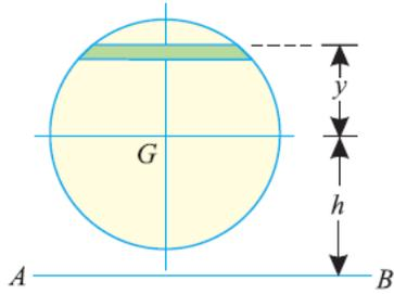
**Proof:** Consider a strip of a circle, whose moment of inertia is required to be found out about a line AB as shown in Fig. Let  $\delta a$  = Area of the strip  $y$  = Distance of the strip from the centre of gravity the section and  $h$  = Distance between centre of gravity of the section and the axis AB. We know that moment of inertia of the whole section about an axis passing through its centre of gravity,  $I_G = \sum \delta a \cdot y^2$
