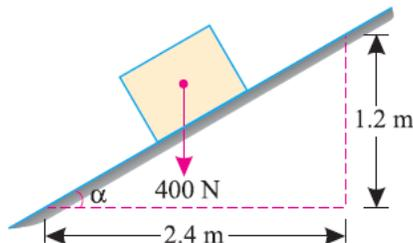
Data Given: Weight of the body ( $W$ ) = 400 N and coefficient of friction ( $\mu$ ) = 0.3.
