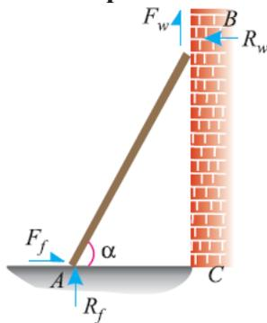
**Q. A uniform ladder of length 3.25 m and weighing 250 N is placed against a smooth vertical wall with its lower end 1.25 m from the wall. The coefficient of friction between the ladder and floor is 0.3. What is the frictional force acting on the ladder at the point of contact between the ladder and the floor? Show that the ladder will remain in equilibrium**
