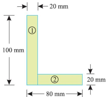
Let left face of the vertical section and bottom face of the horizontal section be axes of reference.
