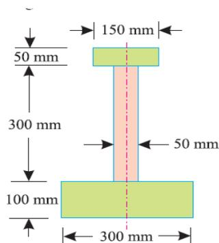
As the section is symmetrical about Y-Y axis, bisecting the web, therefore its centre of gravity will lie on this axis. Now split up the section into three rectangles as shown in Fig. Let bottom of the bottom flange be the axis of reference.
