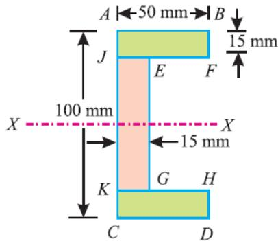
As the section is symmetrical about  $X-X$  axis, therefore its centre of gravity will lie on this axis. Now split up the whole section into three rectangles  $ABFJ$ ,  $EGKJ$  and  $CDHK$  as shown in Fig.
