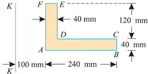
As the moment of inertia is required to be found out about the axis K-K,
