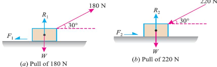
Now consider a push of 220 N acting on the body. We know that in this case, the force of friction ( $F_2$ ) will act towards right as shown in Fig. (b).
