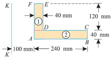
We know that moment of inertia of section (1) about its centre of gravity and parallel to axis K-K is  $I_{G1} = \frac{120 \times 40^3}{12} = 640 \times 10^3 \text{ mm}^4$
