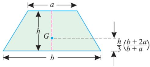
The centre of gravity of a trapezium with parallel sides  $a$  and  $b$  is at a distance of  $\frac{h}{3} \cdot \frac{(2a+b)}{(a+b)}$  measured from the side  $b$
