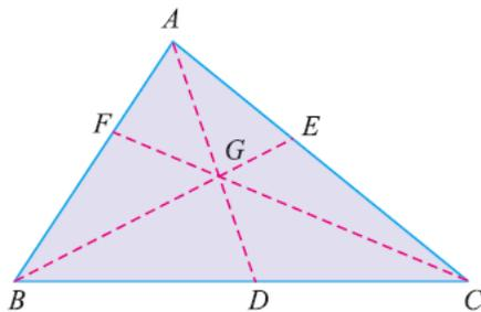
The centre of gravity of a triangle is at the point, where the three medians (a median is a line connecting the vertex and middle point of the opposite side) of the triangle meet
