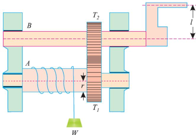
In single purchase crab winch, a rope is fixed to the drum and is wound a few turns round it. The free end of the rope carries the load  $W$ . A toothed wheel A is rigidly mounted on the load drum. Another toothed wheel B, called pinion, is geared with the toothed wheel A as shown in Fig.
