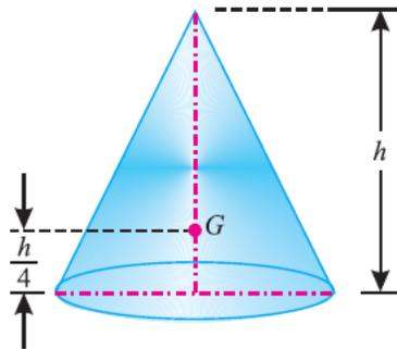
The centre of gravity of right circular solid cone is at a distance of  $\frac{h}{4}$  from its base, measured along the vertical axis
