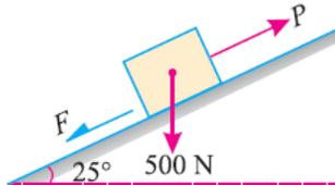
Data Given: Weight of the body ( $W$ ) = 500 N ; Angle at which plane is inclined ( $\alpha$ ) =  $25^\circ$  and angle of friction ( $\phi$ ) =  $20^\circ$ .
