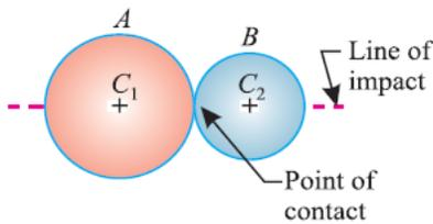
The line of impact, of the two colliding bodies, is the line joining the centres of these bodies and passes through the point of contact or point of collision. If the two bodies, before impact, are moving along the line of impact, the collision is called as direct impact.
