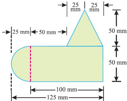
As the section is not symmetrical about any axis, therefore we have to find out the values of both  $\bar{x}$  and  $\bar{y}$  for the lamina.
