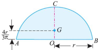
The centre of gravity of a semicircle is at a distance of  $\frac{4r}{3\pi}$  from its base measured along the vertical radius
