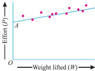
Here the intercept  $OA$  represents the amount of friction present in the machine. The machine friction may be expressed either on the effort side or on the load side. **If expressed on the effort side, the friction may be defined as an additional effort required to overcome the frictional force. But if expressed on the load side, the friction may be defined as the additional load that can be lifted or the additional resistance that can be overcome.**
