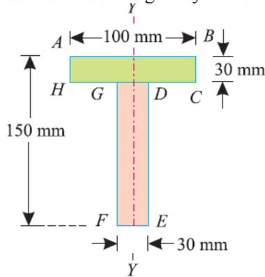
As the section is symmetrical about Y-Y axis, bisecting the web, therefore its centre of gravity will lie on this axis. Split up the section into two rectangles ABCH and DEFG as shown in Fig.
