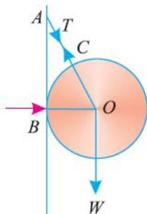
If length of the string  $AC$  is equal to radius of the sphere, find tension ( $T$ ) in the string and reaction of the wall.
